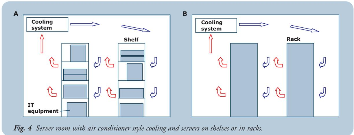
*Fig. 4 Server room with air conditioner style cooling and servers on shelves or in racks.*
