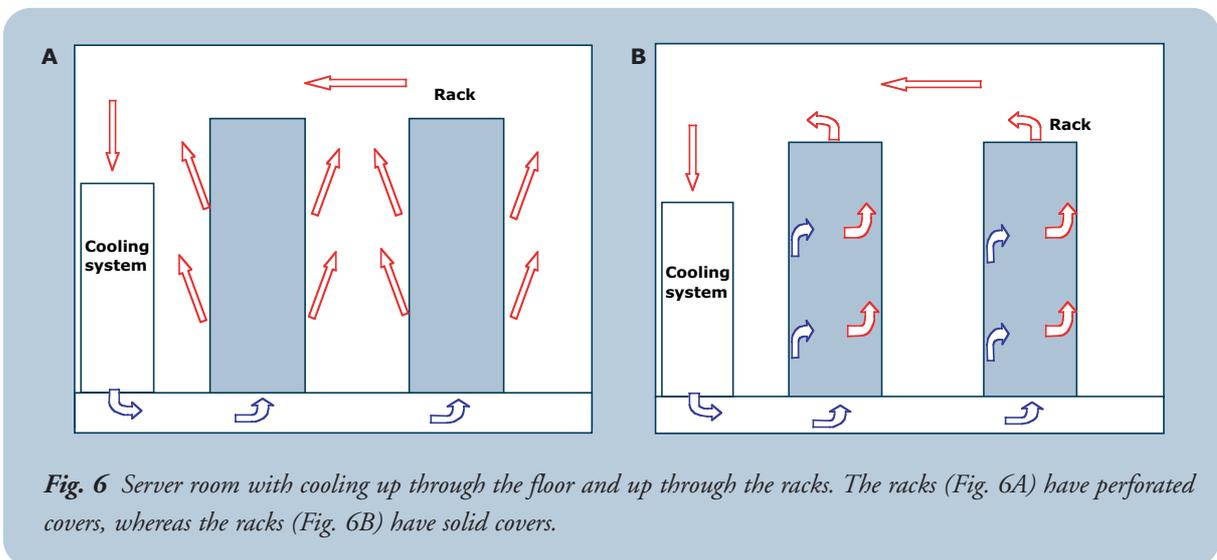
*Fig. 6 Server room with cooling up through the floor and up through the racks. The racks (Fig. 6A) have perforated covers, whereas the racks (Fig. 6B) have solid covers.*
