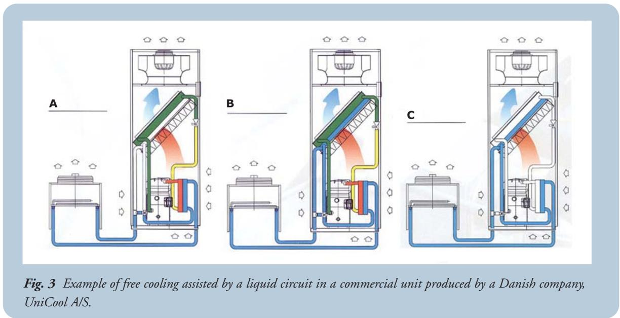
*Fig. 3 Example of free cooling assisted by a liquid circuit in a commercial unit produced by a Danish company, UniCool A/S.*
