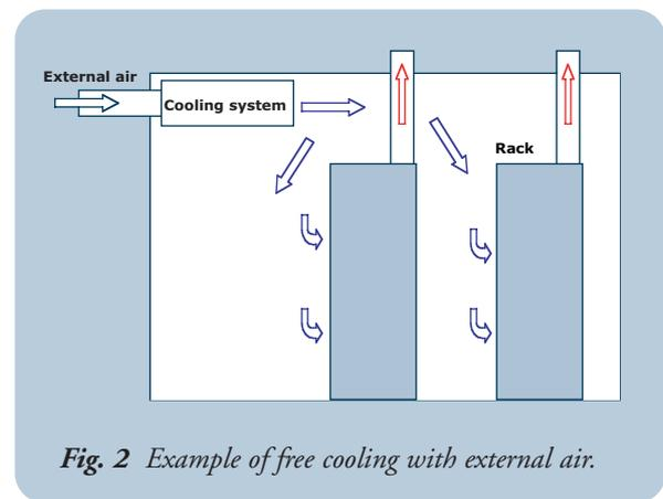
*Fig. 2 Example of free cooling with external air.*
