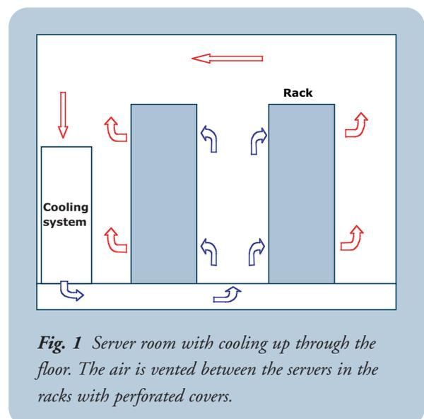
**Fig. 1** Server room with cooling up through the floor. The air is vented between the servers in the racks with perforated covers.
